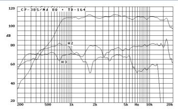
Note: on axis frequency response measured with CP385/Nd standing on infinite baffle in anechoic chamber, 1w @ 1m.
