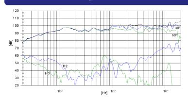
Note: Filtered frequency response measured with loudspeaker standing on infinite baffle in anechoic chamber, 1W @ 1m with
