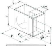
External dimensions for recommended volume, using MDF 19mm (3/4") thick. If the panels are thicker, the difference must be added to these dimensions.
