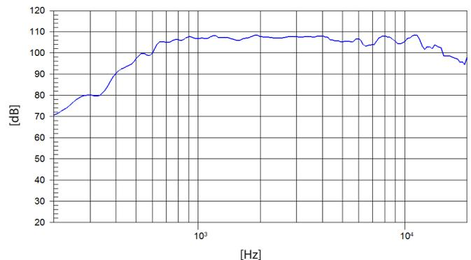
**Note:** On axis frequency response measured coupled to TD-385 horn in anechoic chamber, 1W / 1m
